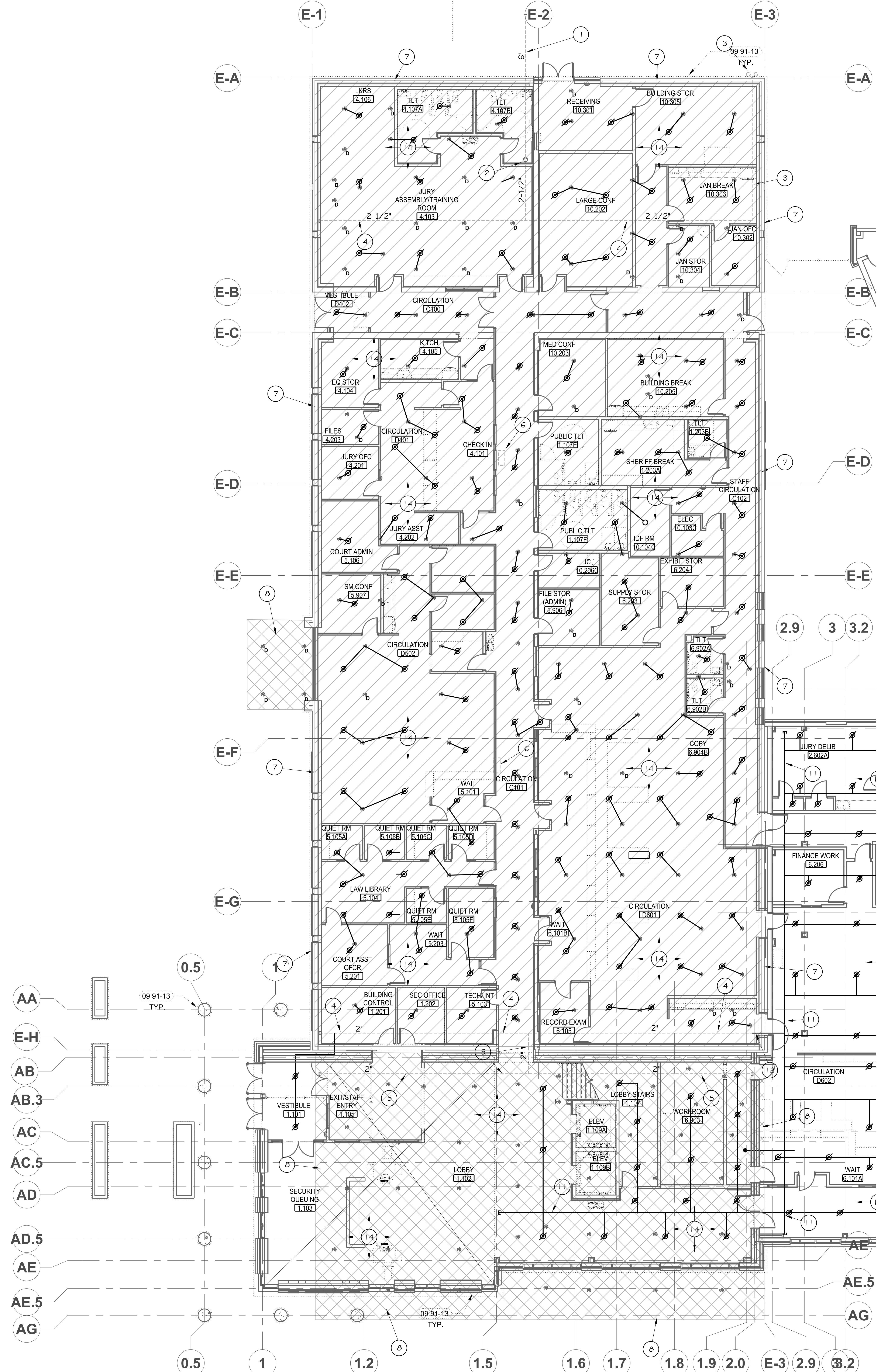
1 FIRE SPRINKLER PLAN - LEVEL 1 AREA A 1/8" = 1'-0"
